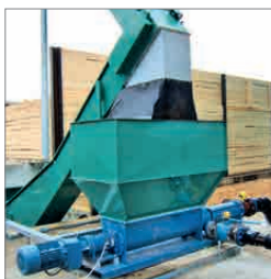
Feeding the pump via a transferring hopper
