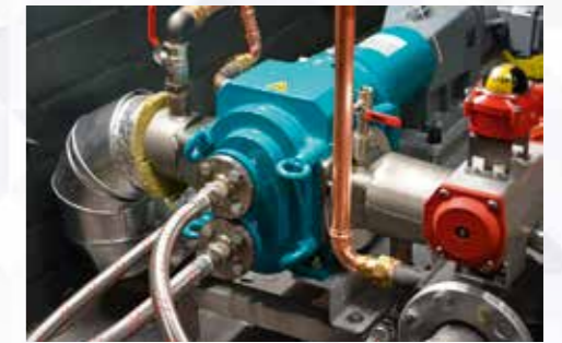
BLUeline pump with heater jacket and heater cover
